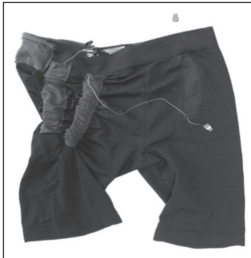
Figure 3 Illustrative screenshot to visualize the concept of ambulant anti-dislocation alarming system following total hip arthroplasty
