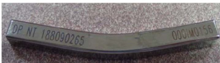
Figure 1. Square, anatomically shaped NiTi alloy Spinal Rod.
