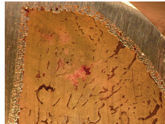
Figure 6 | Enlargement of area directly under the cup. Notice bone trabeculae running in the direction of the porous coating of the cup
