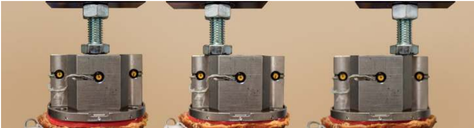
Figure 4. Front view of top-loading on a tensile testing machine via a central and 2 eccentric (medial/lateral) positions (bone/implant perspective).
