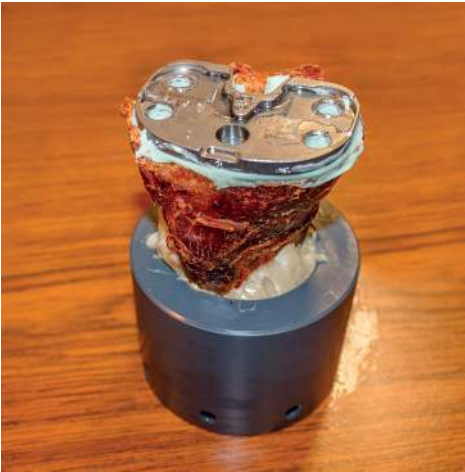
Figure 1. Front-top view of the test-object (polyvinyl-chloride cylinder filled with epoxy resin fixating a right-sided cadaveric tibiae including the tibial tray).
